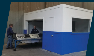
HVAC Climate Room <130°F / 85% Humid.
