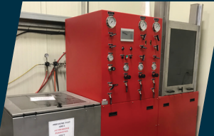
Hydraulic & Gaseous Pressure Testing
