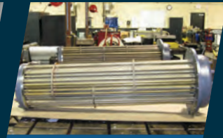
Heat Exchanger Retubing & Repair
